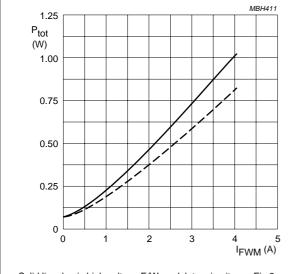
Solid line: basic high-voltage E/W modulator circuit; see Fig.8. Dotted line: basic conventional horizontal deflection circuit; see Fig.9. Curves include power dissipation due to switching losses.
